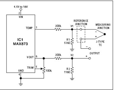
Using voltages generated at TEMP and VOUT by the voltage-reference IC, this circuit compensates the reference junction of a thermocouple.
